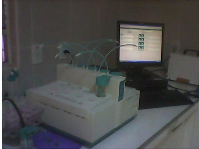
**Figura 14:** Metrohm 873 Biodiesel Rancimat<sup>®</sup>
